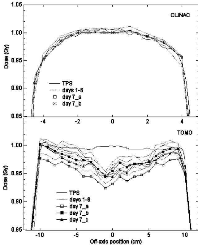
Fig. 7. Typical output variations as observed with a  $10 \times 10 \text{ cm}^2$  reference field on a Clinac (6 MV) and with the cylindrical dose delivery on the TomoTherapy unit. For each treatment unit, day to day (days 1–6) as well as successive measurements on the same day (day 7\_a, day 7\_b, ...) are displayed.
