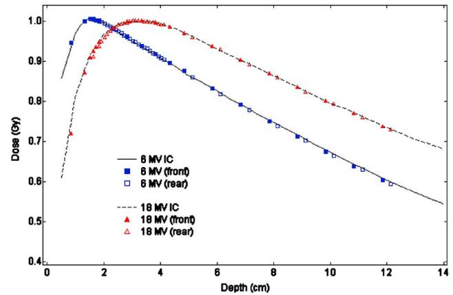
FIG. 3. Absolute depth dose measurements obtained for a  $10 \times 10$  cm<sup>2</sup> field with a single ion chamber in water [solid (6 MV) and dashed (18 MV) line] (SPD=100 cm, 100 MU). Data measured with the central ion chamber of the 2D array in solid water were shifted and renormalized to coincide with the absolute measurements in water. Filled and open markers correspond to array irradiation from the front and from the rear, respectively.
