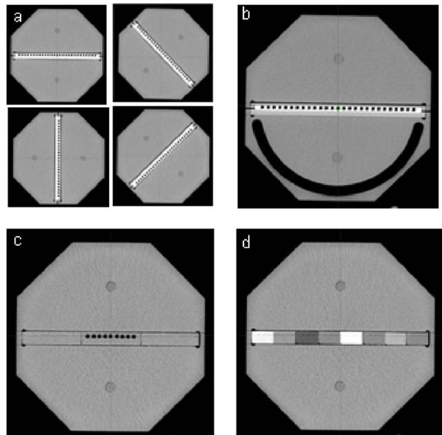
FIG. 1. Different configurations of the Octavius phantom: (a) Octavius<sup>CT-IC</sup> with 2D array for dose calculation in different planes of measurement, (b) Octavius<sup>729</sup>/2D array tandem for measurements, (c) Octavius<sup>CT-IC</sup> with multiple ion chamber insert, and (d) Octavius<sup>CT-IC</sup> with heterogeneous inserts.
