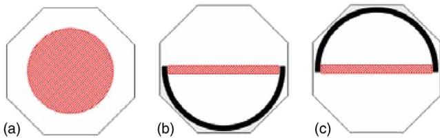
FIG. 2. Schematic of the structures used for generating the TomoTherapy test plans. The circular structure in (a) is used to generate a uniform, cylindrical dose delivery. When optimizing on the rectangular PTV (b) and (c), the half cylinders are used as directional blocks, i.e., to avoid beam delivery from (b) the rear and (c) from the front.
